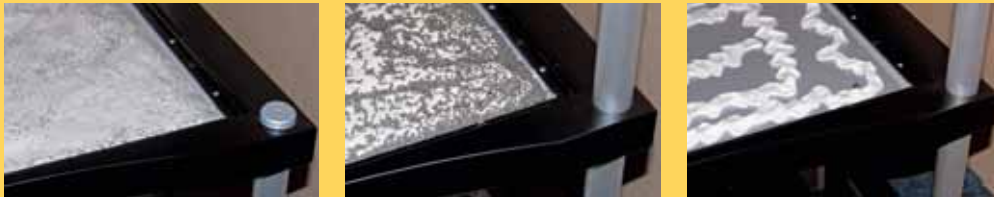
The sound changes according to the filling. It was even audible if the sand/steel ball mix stayed in the plastic bag (left) or was poured out (center). On the right with "terostat".
